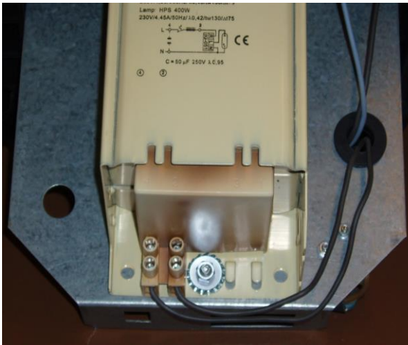
Fig. 2 A choke showing a change in the color of the cover due to increased temperature
